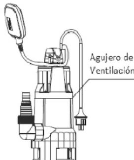
**Note:** The position of the outlet hole may be different depending on which models. The main power cables must not have a smaller cross-section than the rubber sheathed cables with the designation H05RN-F and the designation H07RN-F.
