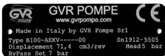
Fig. 202 – Typical nameplate for pump without electric motor
