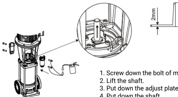
1. Screw down the bolt of mechanical seal.
