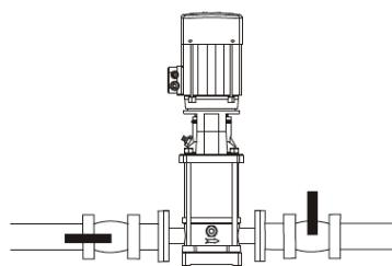
2. Open the priming plug and fill the water.
