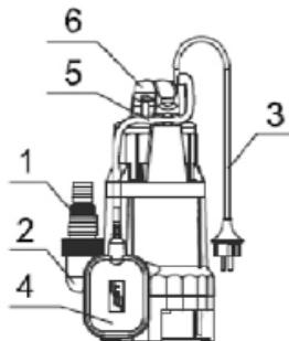
The cable length between the level switch (4) and the level switch lock (5) shall always be at least 10 cm.
