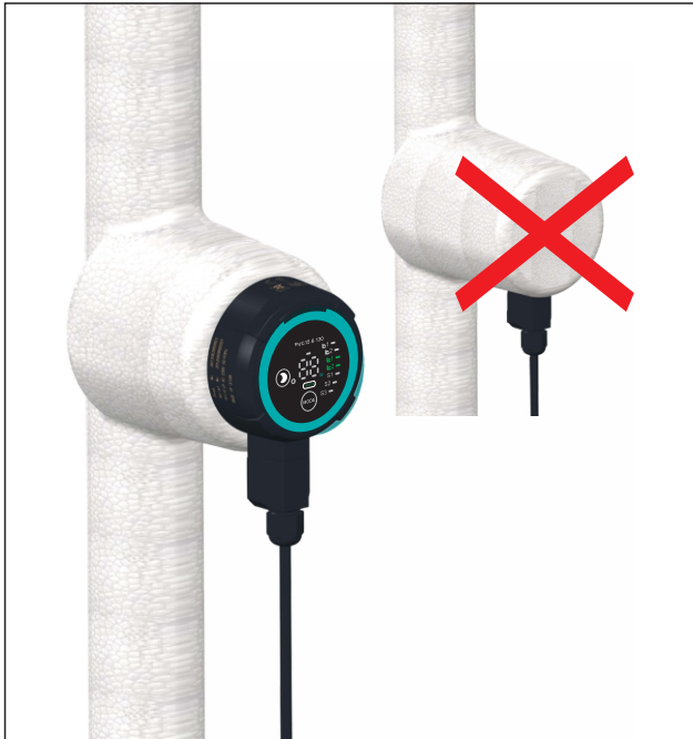
(Pump casing thermal insulation)
