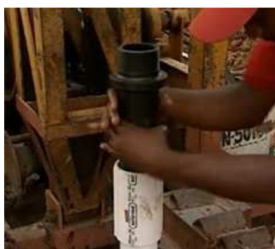
Finish by screwing on the top adaptor.
