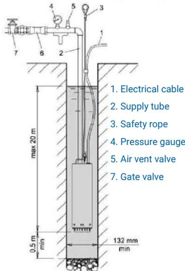
The pump can be kept in a suspended position by the metal supply pipe. Tighten the threaded joints of the pipes securely to prevent loosening during operation.
