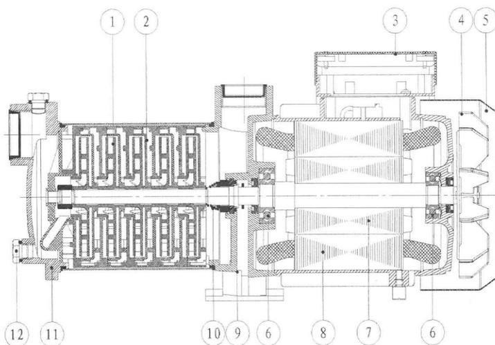
Impeller 3. Junction box 5. Fan cover 7. Rotor 9. Suction casing 2. Diffuser 4. Fan 6. Bearings 8. Stator winding 4. Fan 6. Bearings 10. Mechanical seal 12. Discharge plug
